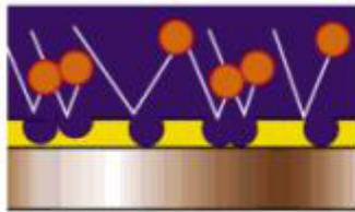
Operating mix too coarse (too much new abrasive added at once)
