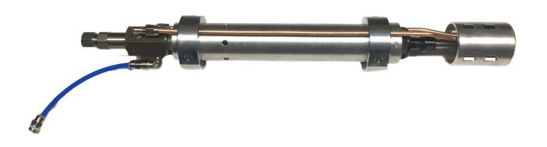
PIPECOATER-III/125 tool is designed to coat the inside of pipe or tubing ranging from 76 to 125 mm (3" - 5") ID without the need to rotate pipe or tubing and to apply an even paint film thickness throughout. Generally, any type of coating may be used in this tool that can be airless sprayed.
