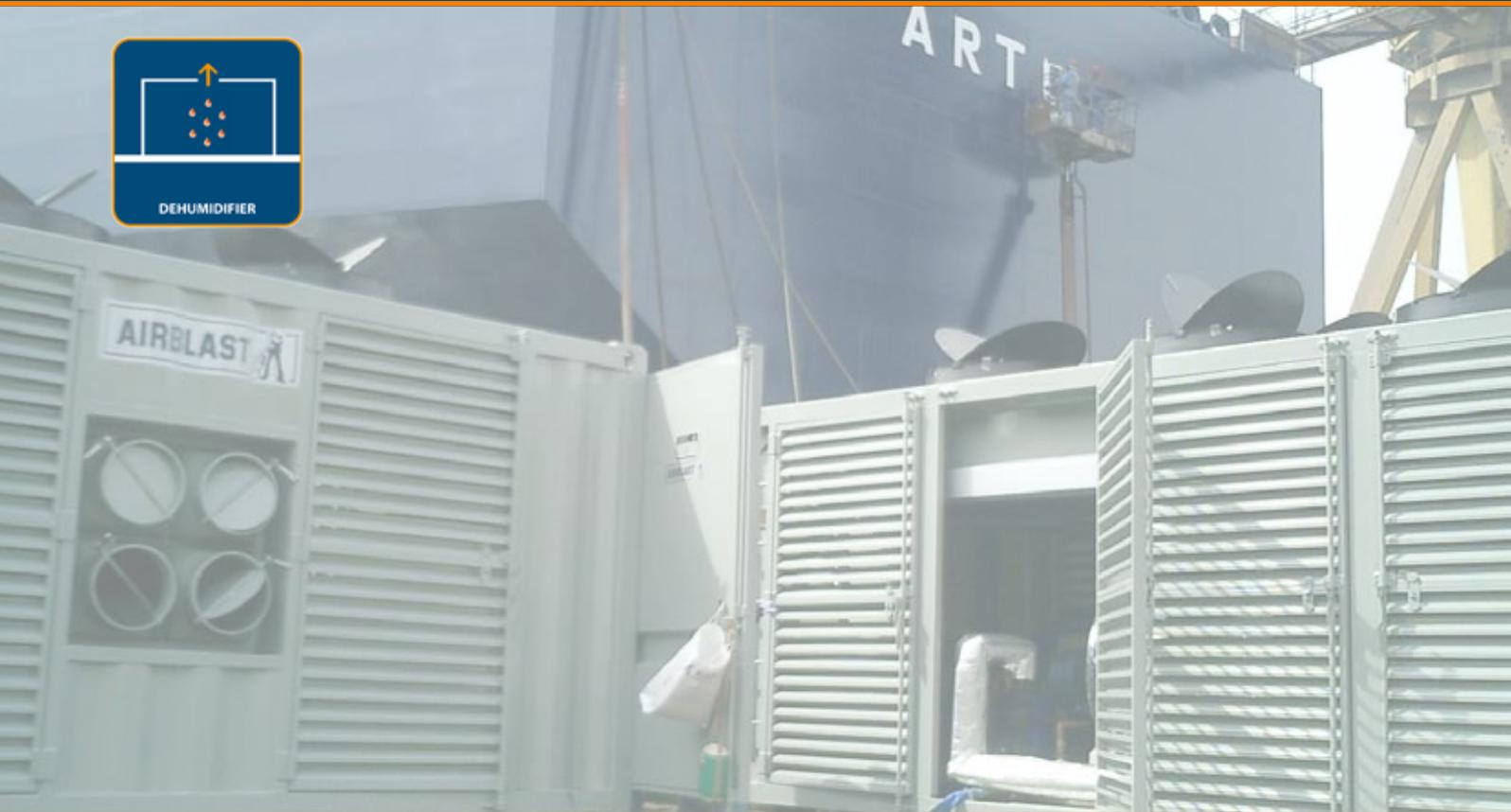
Rust is the enemy of newly blasted steel - high atmospheric humidity coupled with low steel temperatures provide the optimum conditions for the condensation of moisture onto the newly blasted surface. Condensation rust is one of the leading causes of premature coating failure. The Airblast range of dehumidifiers are designed to provide the optimum climatic conditions for blasting by reducing the relative humidity.
