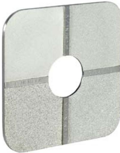
A precision Nickel Comparator Plate that conforms to International Standard ISO 8503 and ASTM D4417 for grit and shot blasted surface roughness comparison.
