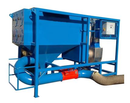
Mobile "explosion proof" cartridge dust-filteruint suitable for dust-extraction during metallization with 85/15 zink/ aluminium wire or 100% zink made of steel sheet 3 mm reinforced with steel profiles.
