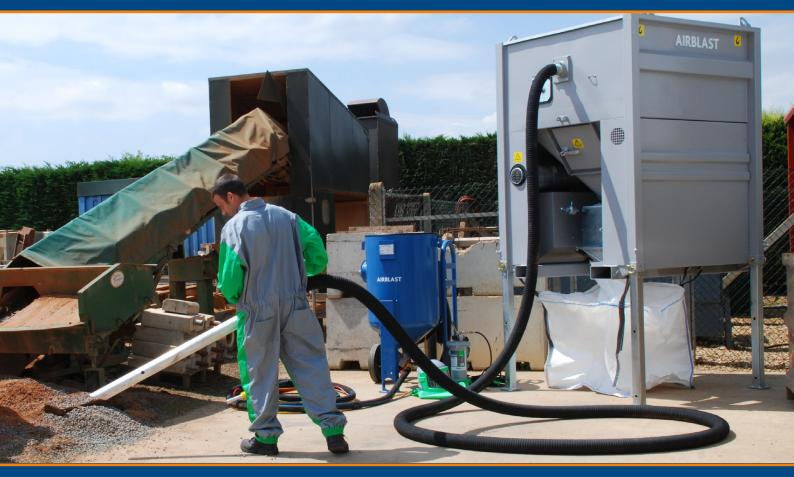
ABVAC is an electric-powered suction unit mounted onto a rigid stand equipped with retractable legs. The unit is designed for the collection of anything from dust up to 50mm debris into a big bag and is ideal for both mobile use and for fixed installations. The unit can also be combined with an abrasive storage hopper to allow recovered abrasive to be reused.
