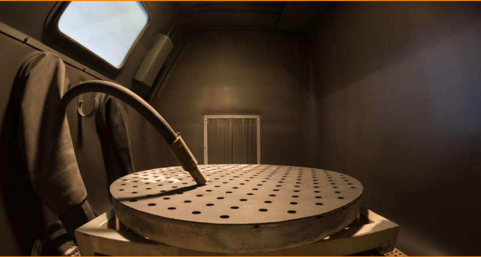
Blast cabinets can be used to blast clean relatively small substrates of surface rust and contaminants in a dust free environmentally friendly manner. Airblast has a complete range of systems which set the standard for optimum performance in modern blast cabinets. Whether you wish to de-burr, clean, remove an existing coating, or produce a matt / polished surface on your substrate an Airblast blast cabinet is the most professional, cost effective equipment available.
