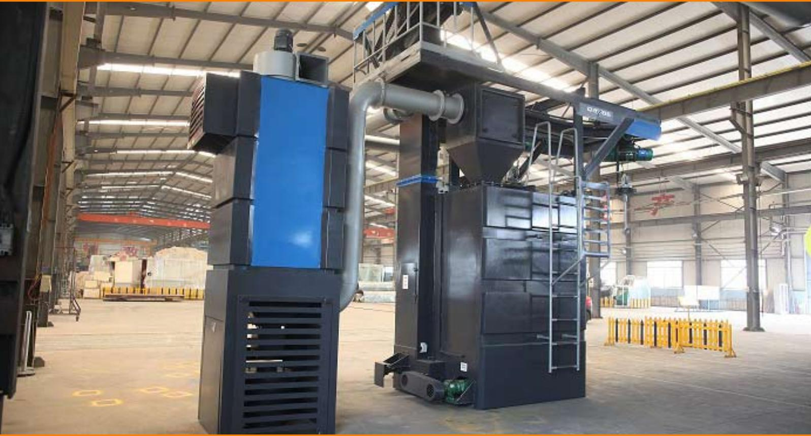
Shot Blasting Machines utilize multiple spinning blast wheels as opposed to air pressure to propel abrasive onto the substrate. As the spinning blast wheels are fixed in place each machine is designed to blast a certain substrate shape in the optimum way. The production characteristics of each wheel blast machine is determined by the quantity, power, and size of the spinning blast wheels.
