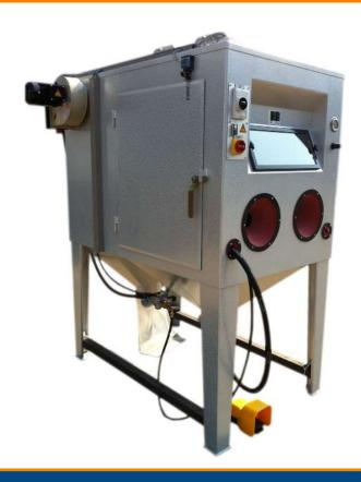
The Airblast Vacuum Injection Cabinets are designed for rust removal, cleaning, slagging, frosting, chipping and polishing. The unit is especially designed for manual blasting of all sorts of smaller items.
