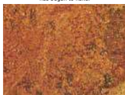
Mill scale on steel surface has rusted away, but with slight pitting visible under normal vision.
