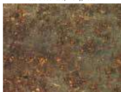
Steel surface has begun to rust and mill scale has begun to flake.
