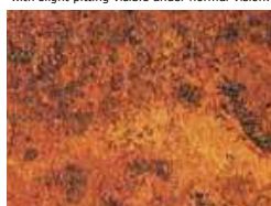
Mill scale on steel surface has rusted away, general pitting is visible under normal vision.
